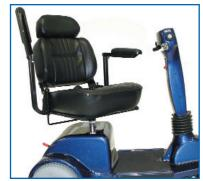
Swing back armrest and swivel seat helps the operator get in and out of the scooter with ease.
