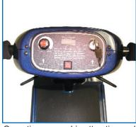
Operating counsel is attractive and easy to read. With **SMART** LCD battery indicator it accurately tells the remaining charge.
