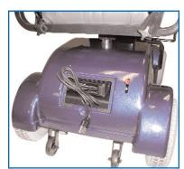
Built in battery charger eliminate the trouble of carrying a separate charging unit.
