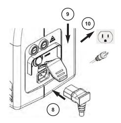
**NOTE:** Check and ensure the pump unit is suitable for the local power voltage.
