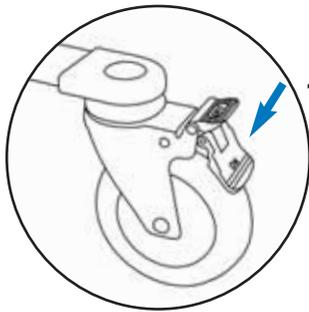
1. Set the unit on the floor. Lock both rear casters to prevent the base from sliding before lifting up the mast.
