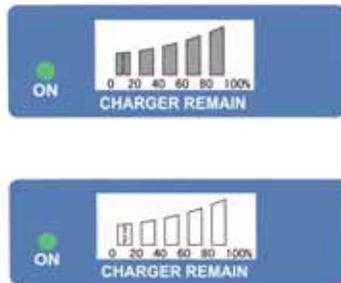
When the battery reserve reaches a desirable level the battery meter stops flashing and the LED turns from red to green. Now the battery meter will indicate a full gauge when all the bars light up. At this time the charger utilizes a slow charging “Absorption Charge”, leave charging for 4 to 6 hours.
