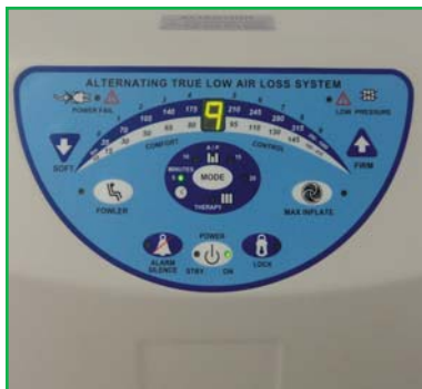
Digital blower based pump is controlled by a micro-processor which allows the caregiver total control over comfort for patient's chosen therapy.
