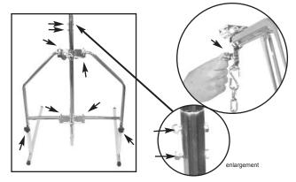
Confirm height and holder settings, and that they are appropriate. Then tighten them. Check all bolts to make sure that they are all tightened. Bolt check points are shown above.
