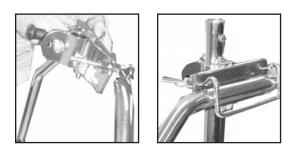
2. Install the top base clamp, ( the one with the extra bar and rubber end cap ). The clamp should be facing down.
