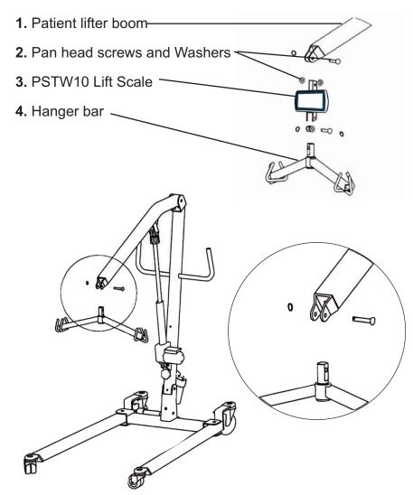
**C.** Insert the hanger bar onto the bottom of the mounting bracket and secure it with a clevis pin, black washers, and a split ring. The screen of the scale faces the front of the lift for easy reading.
