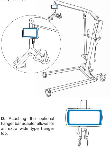
**A.** Remove the hanger bar from the lifter boom (pictured above).
