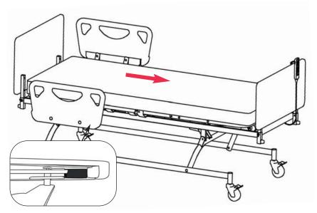
3. Make sure the side with the black release lever faces the foot end of the bed. (Optional 2nd pair of side rail also need to have the lever side face the same direction.
