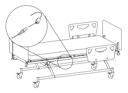
6. Connect the 4 pin round plug into the junction box for built-in back up rechargeable battery.
