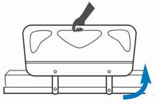
Swing up bed side rail to the upper position, then slide push down to ensure the lock is engaged.
