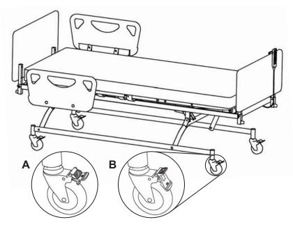
A. Depress the OFF pedal to UNLOCK all four caster wheelsB. Depress the ON pedal to LOCK all four caster wheels
