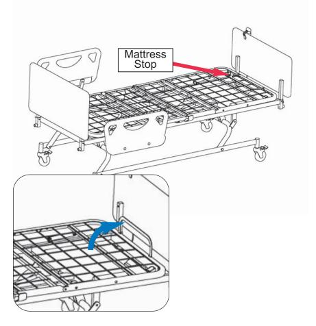
There is one mattress stop located on the end of the bed surface. Flip up the mattress stop and insert the mattress in to hold it in place.
