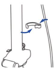
**4c**. Use the included wire clip to secure the loose brake cable.
