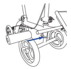
**6c.** Slide the footrest pad onto the other side of the footrest post. Use the footrest pad for rest when leg not paddling.
