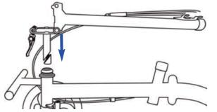
**2a.** Locate the front end of the mainframe and the handle of the scooter. Make sure the screw inside the column lock is loose and completely straight before inserting into front steering column.
