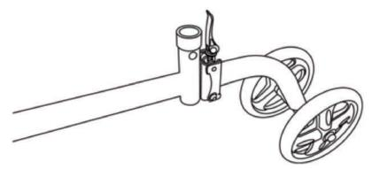
**1c.** Fully extend the frame to straighten, pushing the end into the column lock until the hinge pin clicks in place.
