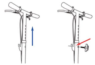
4a. locate the handlebar on top of the steering column post.
