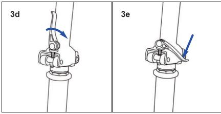
**3d.** Pull the locking mechanism up so that the circular pad rests on top of the steering column folding hinge cutout.
