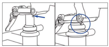
**2b.** Insert the shaft into the steering column. Make sure the back marking pin is lined up with the ridge pockets and that the ledge is pushed down all the way.
