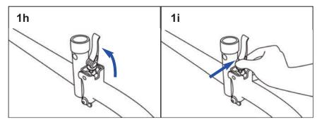
1h. To fold the frame, reverse the procedure in opposite order.1i. Squeeze the frame lever and the side of back frame to disengage the frame locking pin.
