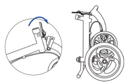
**1a.** Remove all packing materials and set the knee scooter standing along the rear wheels and the leg rest bar.
