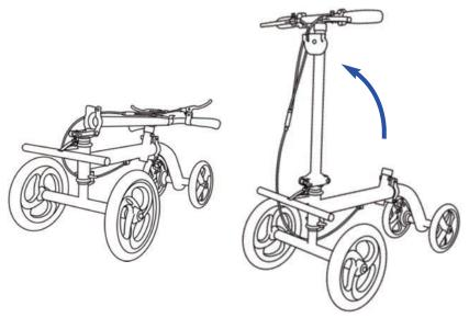
**3a.** Locate the front column lock and lift and straighten the steering shaft until the lock clicks in place.
