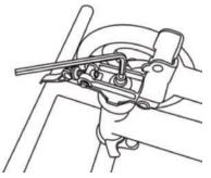
**2c.** Use the allen wrench from the toolkit and tighten the screw inside the lock by turning it clockwise.
