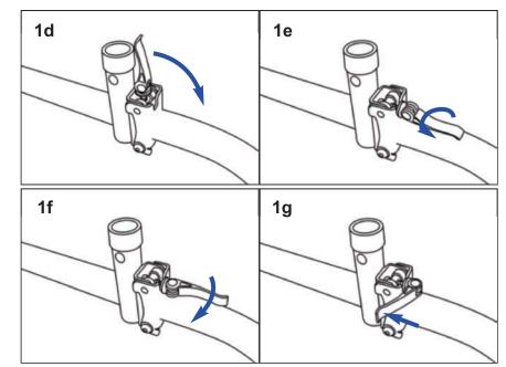
**1d.** Ensure the frame is fully extended and the locking pin is locked into place.
