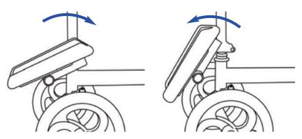
To adjust the angle of the calf leg rest, loosen the heptagon knob found below the pad mount. Adjust to the user's desired level and tighten the heptagon knob to secure position.
