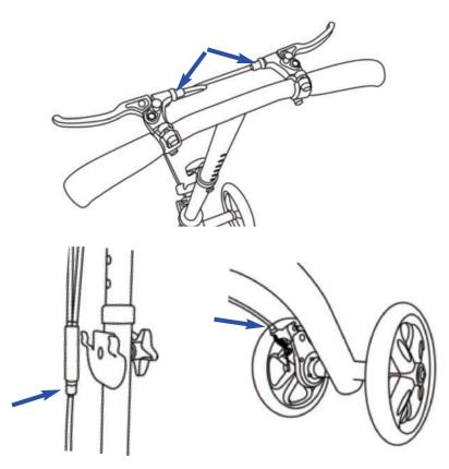
The tightness can be adjusted with the nuts at either end of the brake cable. When adjusting the brake from the brake handle, both sides of the handles should be adjusted to the same tension because they operate the same drum pad.
