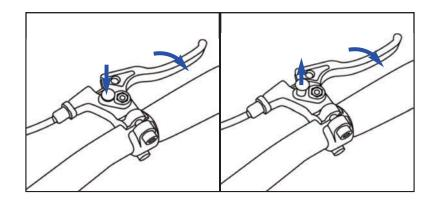
**Setting the locking brake:** squeeze the brake lever and press down the button to engage parking.
