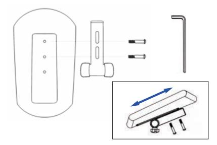
To adjust the extension of the calf leg rest, locate the two screws below the calf pad. Loosen the screws with the allen hex key. Taking off the screw is not necessary for adjustment. Adjust within 1 inch from the normal to extended position. Tighten the screws once finished with adjustments.
