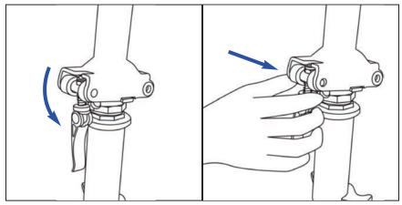
**3f.** To fold the scooter, lift the column lock and pull the lock lever all the way out of the pocket.
