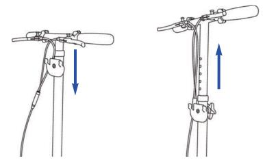
The handle of the knee scooter has multiple holes for height adjustment. Adjust the handle of the scooter to the prefered height by pushing it down pulling it out and secure with the pentagram knob.
