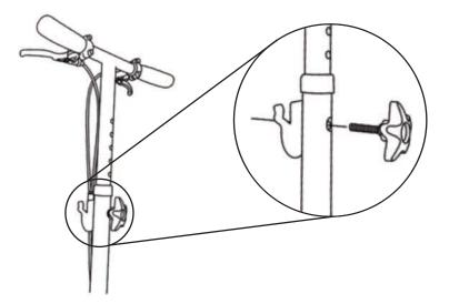
Locate the pentagram knob connecting the handle to the steering shaft and remove it from the steering shaft.
