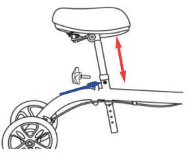
Turn the pentagram knob counter clockwise to remove, extend the platform post shaft up or down to desired height. Align holes in tiller, then insert the pentagram knob screw through the steering tiller. Tighten the pentagram knob by turning it clockwise to secure.
