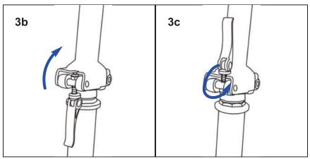
**3b.** Push the steering column upward until it is in a fully upright position.
