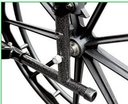
Dual position rear axle easily lowers the seat height by 1 1/2".
